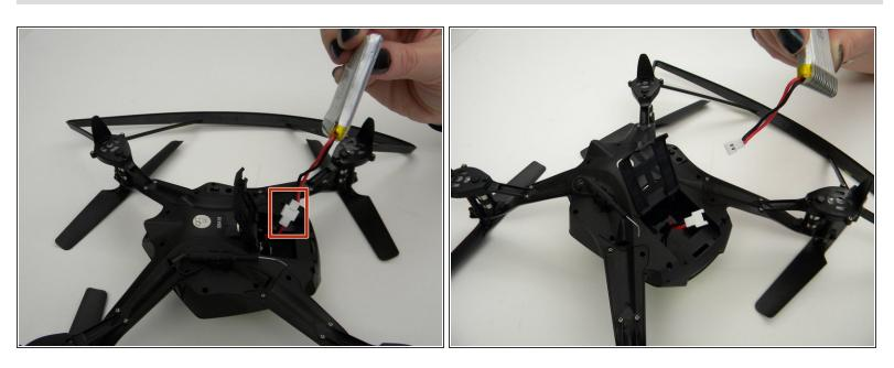
Disconnect white connectors between the battery pack and drone.
