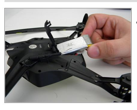
Remove battery pack from body of drone.
