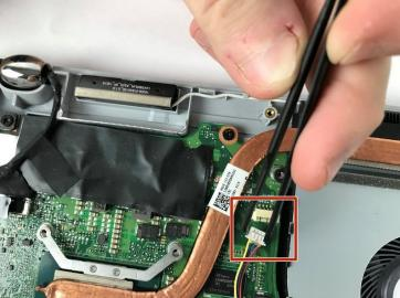
• Use a pair of tweezers to pull and disconnect the cable located to the right of the heat sink fan.
