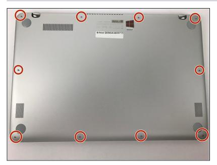
Use the T5 Torx screwdriver to remove the ten 1mm screws located around the back cover.
