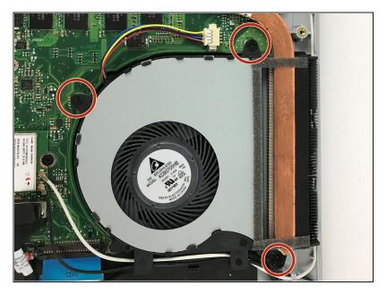
• Using a Phillips #0 screwdriver, remove the three black 4mm screws located around the heat sink fan.
