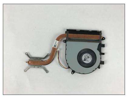
• Remove the heat sink from the device.
