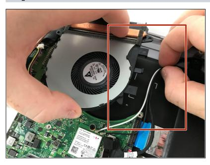
Carefully unravel the cables (two black and one white) to the left of the heat sink fan.
