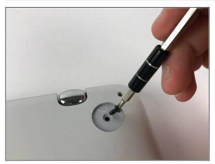
• Use the Phillips #0 screwdriver to remove the two 4mm screws that are under the rubber pads.
