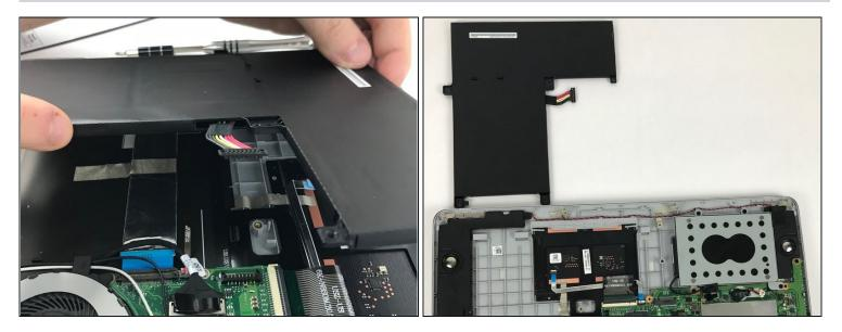
• Remove the battery from the device.
