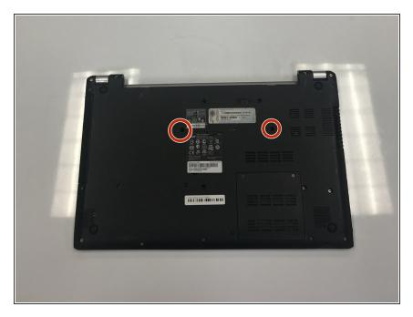
Unscrew the two 8 mm Phillips #0 screws attached to the keyboard.
