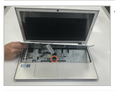
Disconnect the keyboard label connected to the laptop.
