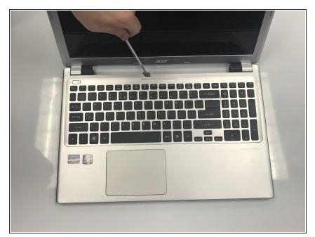
Pry open the keyboard at the top of the keyboard.
