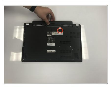
Unlock the battery by pushing the button to the right.
