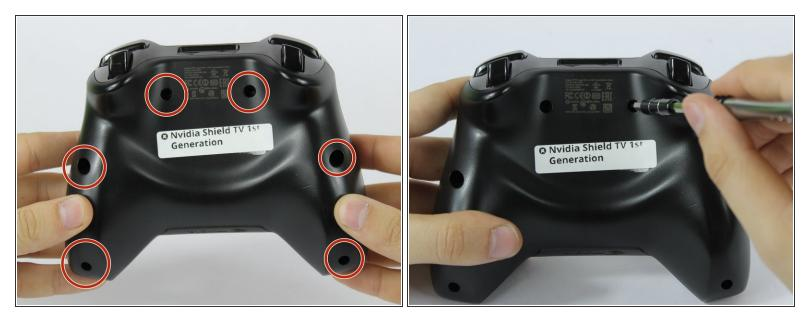
• Remove the indicated six screws using the T6 Torx screwdriver.
