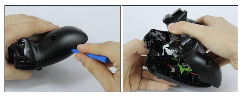
• Use the plastic opening tool to pry the face of the controller from the body.
