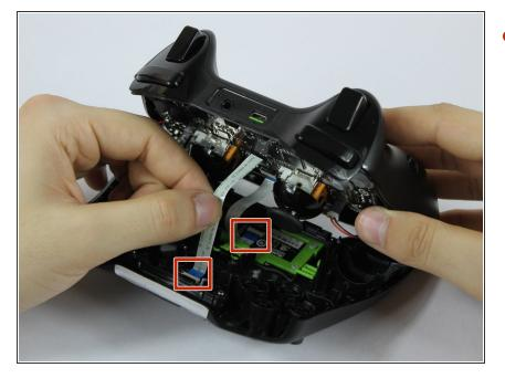
• Carefully remove the indicated ribbon wires from the face of the controller.
