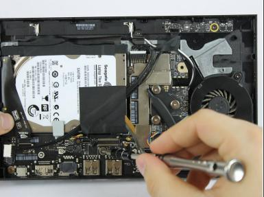
Remove the indicated four screws using the T6 Torx screwdriver.
