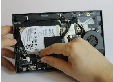
Remove the indicated cables and ribbon wires.
