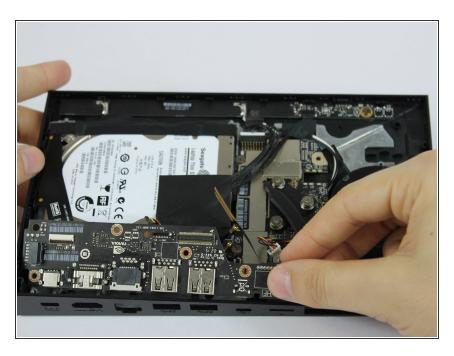
Carefully tilt and pull out the I/O board from the device.
