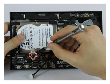
Remove the indicated screw using the T6 Torx Screwdriver.
