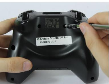
Remove the indicated six screws using the T6 Torx screwdriver.
