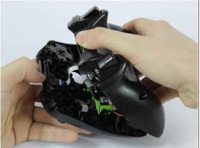
Use the plastic opening tool to pry the face of the controller away from the body.
