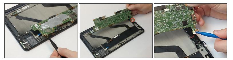
Rotate the motherboard upwards from the tablet using tweezers, but do not remove completely
