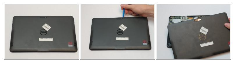
Using the blue opening tool, separate the back plastic cover from the device. Start in a corner, and work your way around the tablet.
