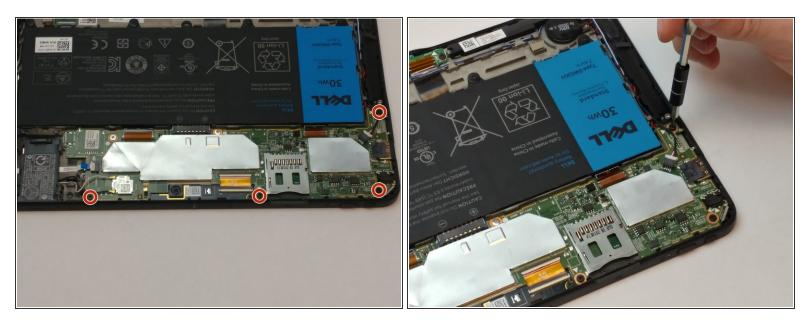
• Remove the four 4.0mm black screws on the perimeter of the device using a JIS #00 screwdriver
