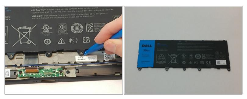
• With the blue opening tool, gently lift up and remove the battery from the tablet.
