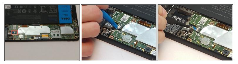
Using an opening tool, lift upwards on the white clamp, and pull the blue tab out of the connection with tweezers.
