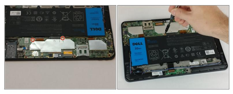
• Remove the two 4.0mm silver screws using the JIS #00 screwdriver.
