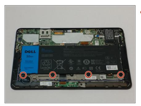
Remove the four 7.0mm screws securing the battery with a JIS #00 screwdriver.
