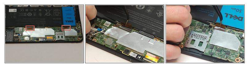
• Disconnect the two clamps, one orange and one white, using tweezers next to the battery.
