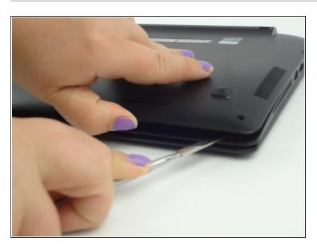
Wedge a metal spudger between the keyboard and bottom cover and slide it around the perimeter until all edges separate.
