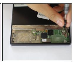
Locate the 3 Phillips screws (PH 0) on the motherboard and proceed to unscrew them using a screwdriver with a PH 0 bit.
