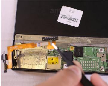
• Use the tweezers to pluck the orange bridge power connector from the Kindle. The charging port and power button is attached to the connector.
