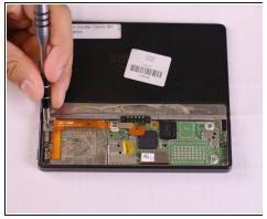
• Locate the 2 Phillips screws (labeled PH 0) and remove screws using a screwdriver with a PH0 bit.
