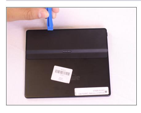
Carefully wedge the plastic opening tool between the back panel and the device to free the clips holding the back panel and the device together.
