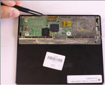
Locate the connector from the display screen on the motherboard and disconnect it with tweezers
