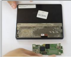
Use the metal spudger to wedge out the motherboard from the Kindle.
