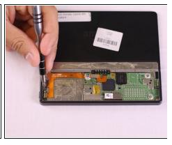
• Locate the 2 Phillips screws (labeled PH 0) and remove screws using a screwdriver with a PH0 bit.
