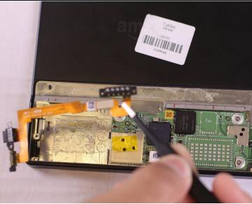
• Use the tweezers to pluck the orange bridge power connector from the Kindle. The power button is attached to the connector.
