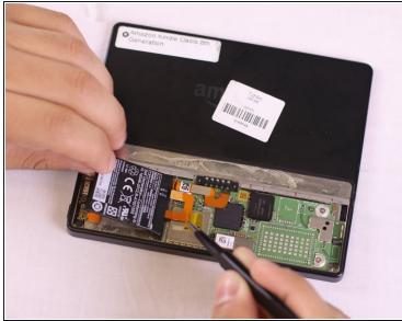
• Using the <u>tweezers</u>, gently lift the tape off of the Power bridge connector. If a new unit comes with a new piece of tape, remove entirely, if not remove and place one corner lightly face down on a clean surface to be used again.
