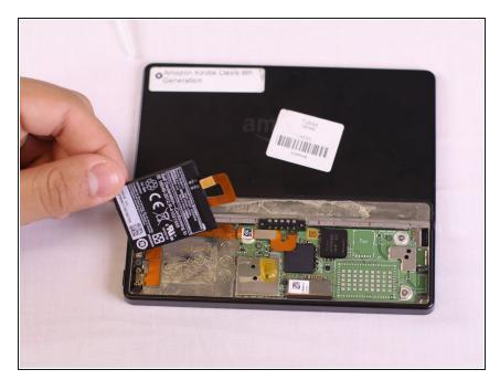
Once free of the adhesive and connectors, remove the old battery from the device.
