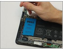
Using aJIS #00 screwdriver locate and remove the two 3.5mm screws by the plastic covers on left and right side of the tablet
