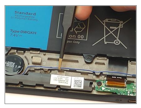
Use tweezers to help lift the white and blue wires connecting both speakers.
