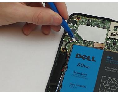
Using the blue opening tool to gently remove the wire connecting the speaker to motherboard
