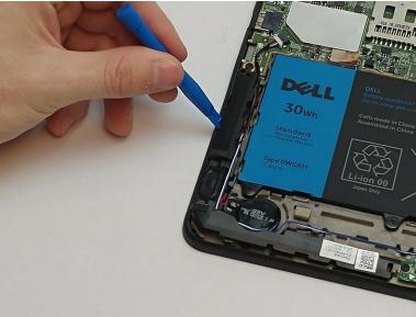
Use the blue opening tool to lift up the speaker counterclockwise from the corner. As you lift up, the speaker will release from the casing. Repeat this process for the second speaker.
