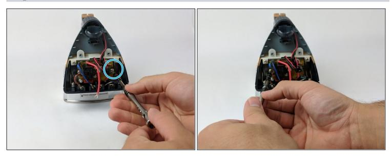
• Remove two screws (left and right) affixed to circuit board.
