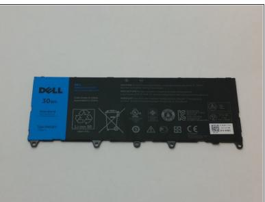
With the blue opening tool, gently lift up and remove the battery from the tablet.
