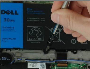
Remove the four 7.0mm screws securing the battery with a JIS #00 screwdriver.
