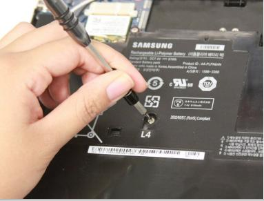
Remove the four 3 mm screws using a Phillips #000 screwdriver.
