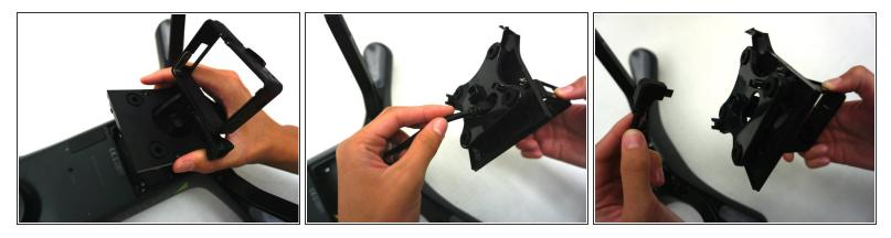
• Once the gimbal and panel is loose enough to pull off with your hand, gently remove both the panel and the gimbal from the device.
