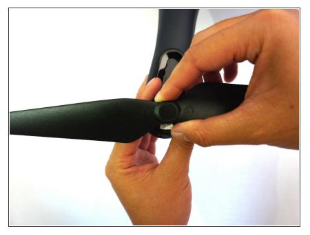
Grip the arm, which is located underneath the propeller, with one hand, and with your dominant hand grip the center of the propeller.
