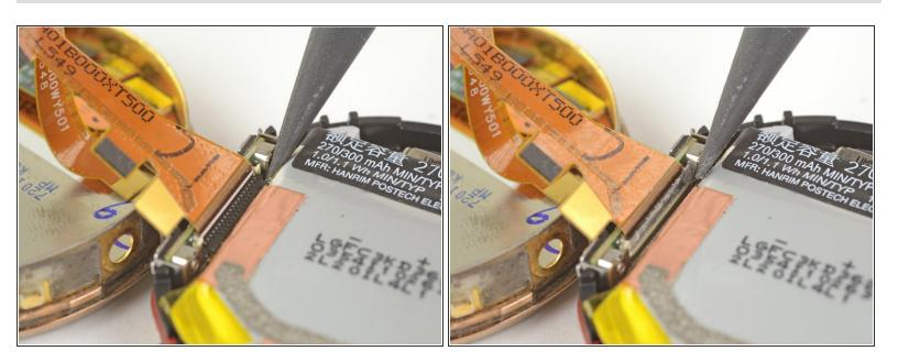
Use a spudger to lift the locking flap on the display ZIF connector.
