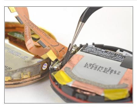
Use tweezers to remove the small rubber strip between the battery and the display ZIF connector.
