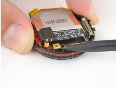
• Use the point of a spudger to pry up the battery connector and disconnect the battery.
