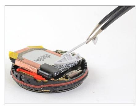
Use tweezers to lift out the grey plastic cover over the battery connector.
