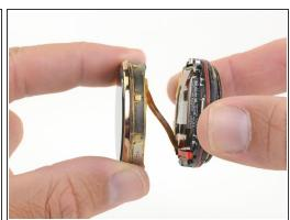
• Use a fingernail or opening tool to pry the plastic lower assembly away from the display assembly.
