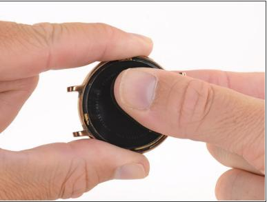
While holding the outer case steady, twist the inner watch assembly clockwise until it stops.
