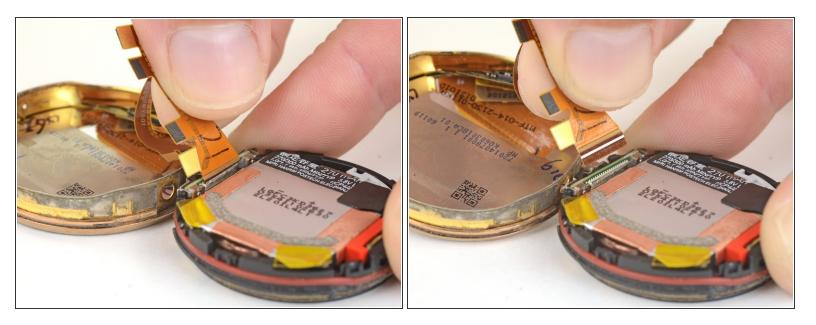
• Lift the display cable straight out of its connector on the motherboard.
