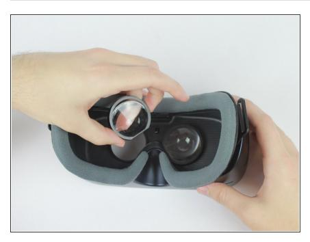
Flip the headgear and use your fingers to gently remove lens from mask. Repeat for both lens.
