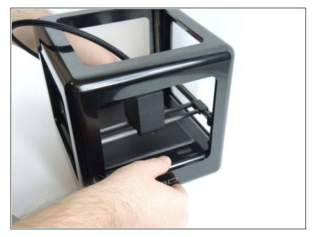
Removing the frame is necessary to access the z axis belt, motors and ports. Make sure the unit is unplugged and set on a hard level surface.
