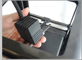
Pull the x-rods away from the plastic sliders on the y-rods, and flip the slider upwards to release the tracks. Lift the extruder assembly out of the way.
