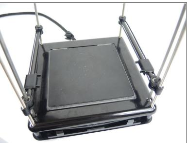
No tools are required to remove the frame. Press down on the printing bed with your thumbs while lifting the frame with your fingers. The frame easily slides up.
