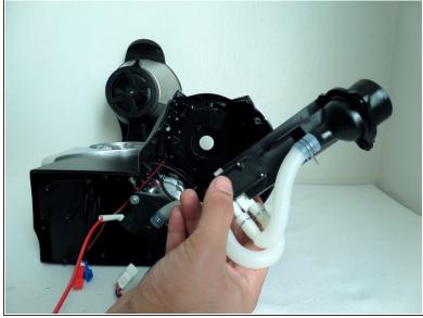
Pull the water tube towards you to detach the water's tube top from the machine.
