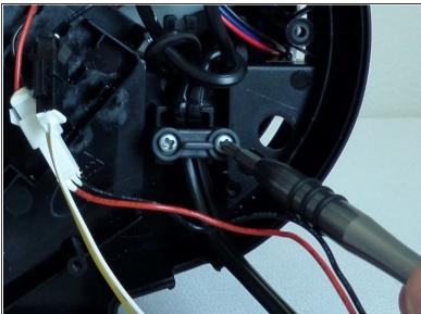
Remove the two 0.6cm with Phillips #2 screwdriver.
