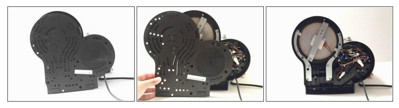
Remove the bottom board with moderate force.
