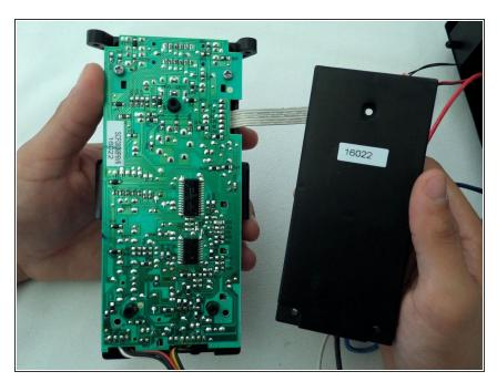
Remove the black board attached to the module.
