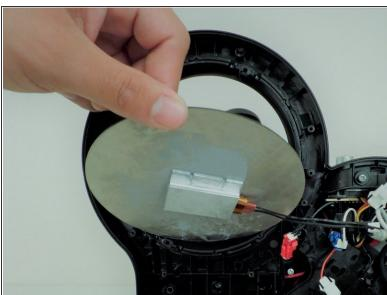
Remove the heated plate from the machine with easy glide.
