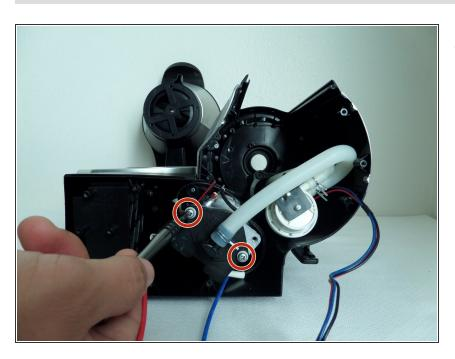
Remove the two 0.8 cm screws with Phillips #1 screwdriver.
