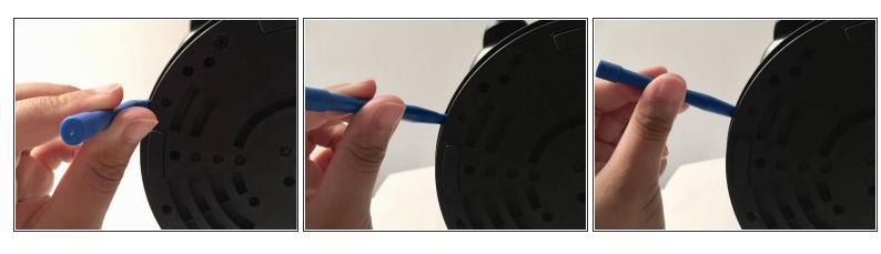
With moderate force remove and place the "plastic opening tool" between the divide in order to remove the bottom board.
