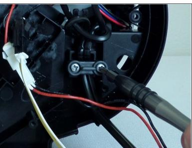
Remove the two 0.6cm with Phillips #2 screwdriver.
