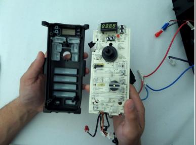
Carefully remove the control panel from the control module.
