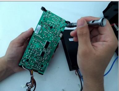
Unscrew four 1.2cm screws with Phillips #2 screwdriver.
