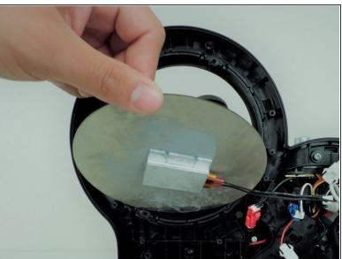
Remove the heated plate from the machine with easy glide.
