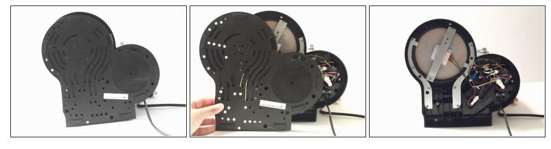
Remove the bottom board with moderate force.
