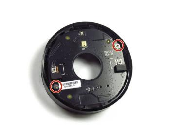
After the cover is removed, unscrew the two Phillips #00 5.0mm screws. Then the board should slide right out.
