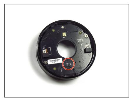
The light sensor is located at the bottom of the board.
