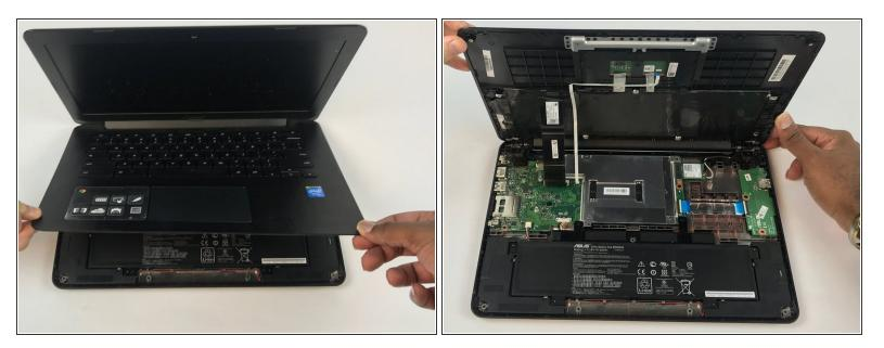
Lift the keyboard panel away from the components at its hinges, which are located at the back of the laptop.
