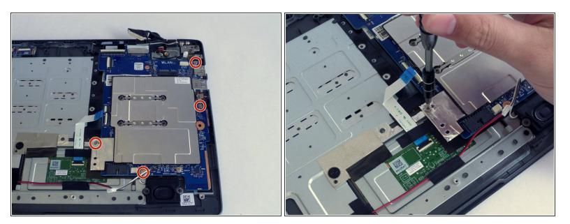
• Remove the four 4-mm screws holding the metallic plate using a PH0 screwdriver.
