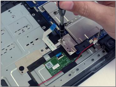
• Remove the four 4-mm screws holding the metallic plate using a PH0 screwdriver.
