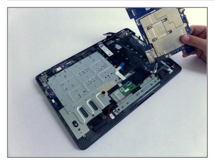
Detach the motherboard by lifting it up and away from the body of the laptop.
