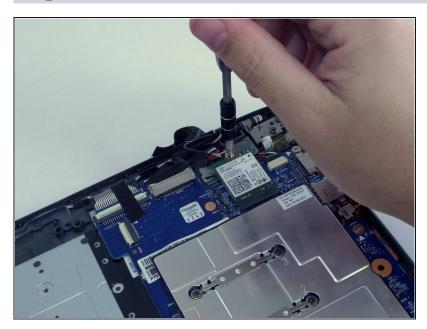
Remove the 3-mm screw that holds the WiFi module to the motherboard using the PHO screwdriver.
