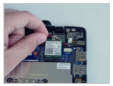
Unplug the white and black wires by lifting them up by hand or using tweezers.
