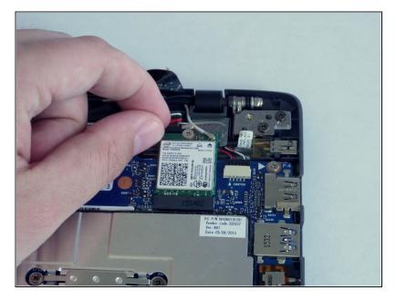
• Unplug the white and black wires by lifting them up by hand or using tweezers.
