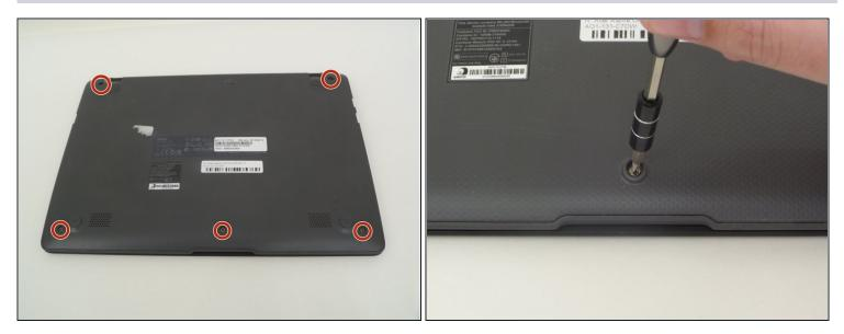
• Unscrew the five 5-mm screws using the PH0 screwdriver.
