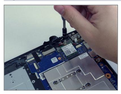
• Remove the 3-mm screw that holds the WiFi module to the motherboard using the PH0 screwdriver.
