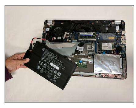
• Lift the battery up and remove.
