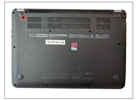
Unscrew and remove the one 7.5 mm Phillips-head screw using Phillips #1 screwdriver.
