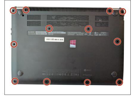
Unscrew twelve 6.0 mm Phillipshead screws using Phillips #1 screwdriver.
