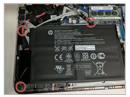
Unscrew and remove the three 4.0 mm Phillips-head screws that hold the battery in place, using a Phillips #1 screwdriver.
