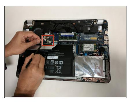
Use the flat end of a plastic spudger to disconnect the battery cable from its socket in the motherboard.
