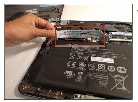
• Once the device is open, move the ribbon cable to the side.
