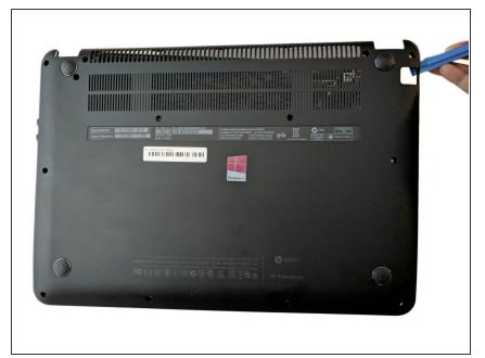
• Use the plastic opening tool (which is short and has a thin end for prying open device parts) to pry open the back case of the device.
