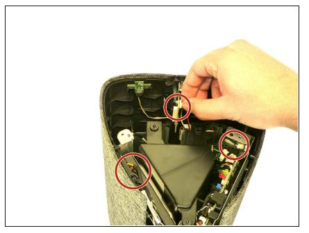
Remove the three wires connecting the outer cover and front I/O port to the internal components (front usb and auxiliary assembly).
