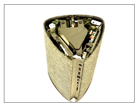
Remove the bottom cover by lifting it up from chassis.
