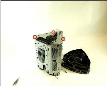
Remove the top bezel from the unit using a Torx Head #15 screwdriver to remove three 24 mm screws and a Phillips Head #00 screwdriver to remove the single 24 mm screw around the outside edge of the chassis.
