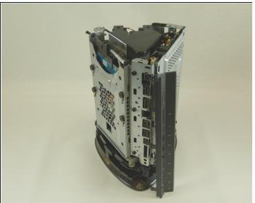
Remove rear I/O bezel using plastic opening tool to pry apart the four clips holding the I/O bezel to the chassis.
