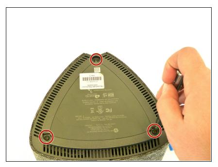
Remove the three 24 mm screws from the bottom cover using a Phillips #2 screwdriver.
