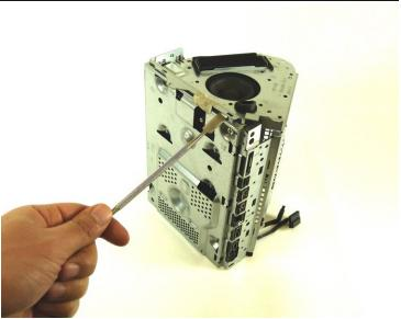
Remove the top chassis cover from the main chassis using the Torx Head #15 screwdriver to remove the nine 24 mm screws and then use the metal prying tool to pry the top chassis cover from the clips holding it to the main chassis and lift carefully away from internal components.
