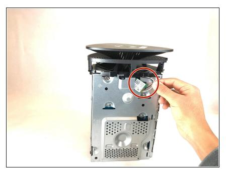
Disconnect the microphone computer chip from the internal components by first peeling away the black adhesive holding the wires to the chassis and gently pulling the chip and wires from its connection.
