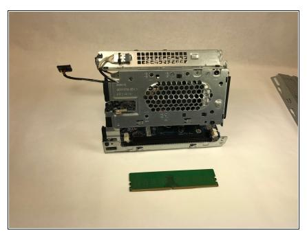
Lift the memory circuit board up and out of its connection, and out of the main chassis.
