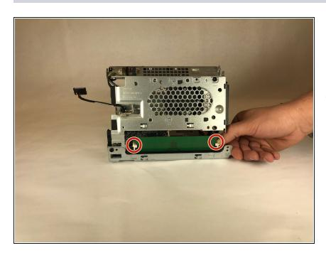
Remove the memory circuit board by pushing down on the white tabs on either side of the memory circuit board until it slightly pops up.
