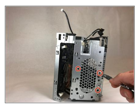
Remove the fan by removing the three 23 mm silver screws that hold the fan to the chassis using a Phillips Head #0 screwdriver.
