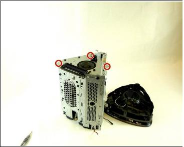
Remove the top bezel from the unit using a Torx Head #15 screwdriver to remove three 24 mm screws and a Phillips Head #00 screwdriver to remove the single 24 mm screw around the outside edge of the chassis.
