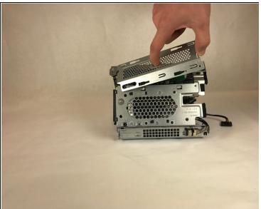
Remove the memory cover by removing the single 24 mm screw holding it to the main chassis using the Torx Head #15 screwdriver and sliding it up and out of its locking clips.
