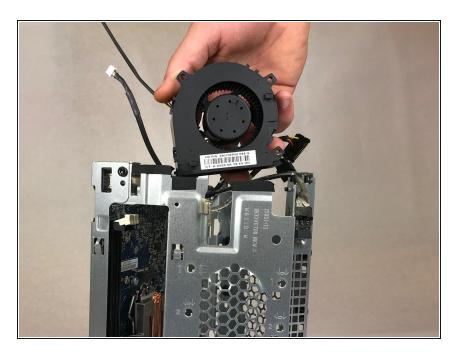
Remove the fan from the chassis by sliding it up and out of the the clips holding the fan to the chassis.
