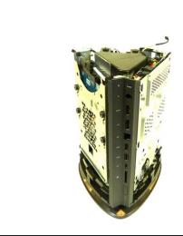
Remove the outer cover by gently pulling apart and pulling away from the chassis.
