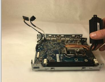
Remove the heatsink from the motherboard by removing three 24 mm screws using the Torx
