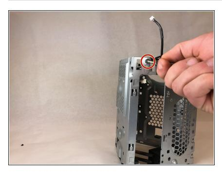
Remove the heatsink from the chassis by using the Philips Head #2 screwdriver to remove two 24 mm screws.
