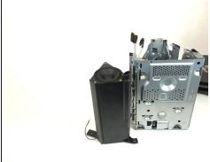
Remove the speaker by removing three 24 mm screws using the Torx Head #15 screwdriver and carefully lifting up and out from internal components.
