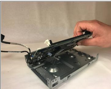
Remove the motherboard from the chassis by removing four 24 mm screws (two on front and two on back) using the Torx Head #15 screwdriver and gently lifting out and away from metal chassis.
