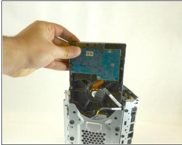
Remove the HDD by first using the Phillips #2 screwdriver to remove the four 23 mm screws holding together the assembly and then pulling the HDD out of the chassis.
