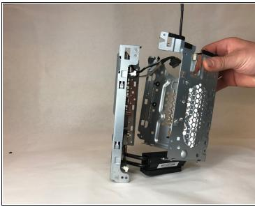
Remove two sides of the chassis from the motherboard and heatsink by removing one 24 mm screw using the Phillips Head #2 screwdriver and three 24 mm screws using the Torx Head #15 screwdriver and gently lifting away from the motherboard.
