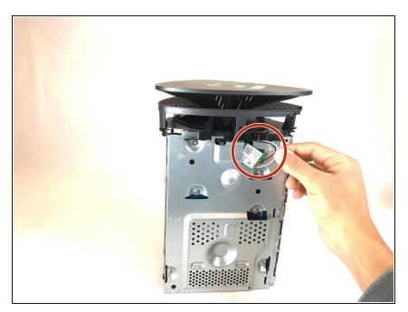
Disconnect the microphone computer chip from the internal components by first peeling away the black adhesive holding the wires to the chassis and gently pulling the chip and wires from its connection.
