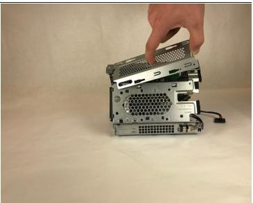
Remove the memory cover by removing the single 24 mm screw holding it to the main chassis using the Torx Head #15 screwdriver and sliding it up and out of its locking clips.
