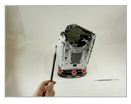
Remove the three 24 mm screws that connect the top cover to the chasis inside the HDD compartment using theTorx #15 screwdriver (an extension and torque lever might be useful).
