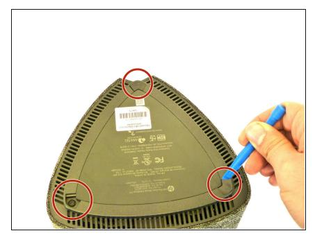
Remove the three rubber footings by prying from the bottom cover using the plastic opening tool.
