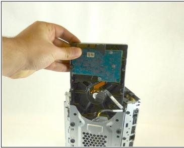
Remove the HDD by first using the Phillips #2 screwdriver to remove the four 23 mm screws holding together the assembly and then pulling the HDD out of the chassis.
