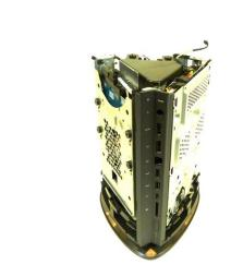
Remove the outer cover by gently pulling apart and pulling away from the chassis.
