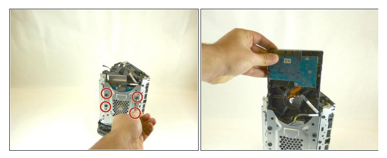
• Remove the HDD by first using the Phillips #2 screwdriver to remove the four 23 mm screws holding together the assembly and then pulling the HDD out of the chassis.
