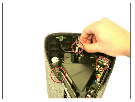
Remove the three wires connecting the outer cover and front I/O port to the internal components (front usb and auxiliary assembly).
