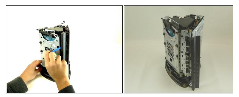
• Remove rear I/O bezel using plastic opening tool to pry apart the four clips holding the I/O bezel to the chassis.
