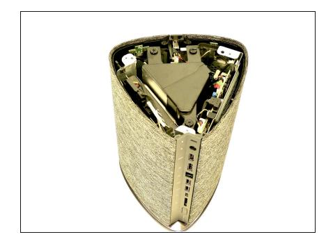
• Remove the bottom cover by lifting it up from chassis.
