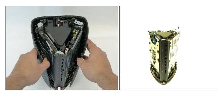
• Remove the outer cover by gently pulling apart and pulling away from the chassis.
