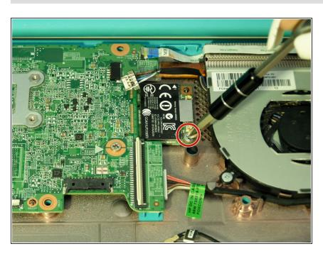
Remove the 3mm screw that holds down the Wifi mini-PCI card using a Phillips Head 1 driver.
