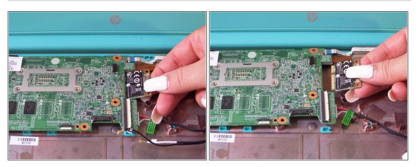
Using your fingers, pull the Wi-Fi card located on the right side of the detached motherboard out of its place.
