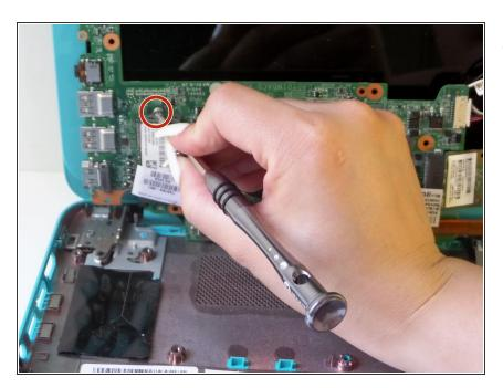
Remove the 3mm screw located directly above the NGFF SSD card using a Phillips Head 1 driver.
