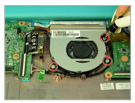
Remove the three 3mm screws that hold the cooling fan in place using a Phillips Head 1 driver.
