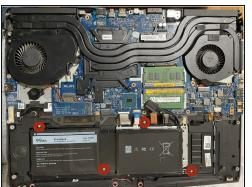
• Unscrew the four M2.5 screws (2.4 mm) with a PH1 screwdriver bit.
