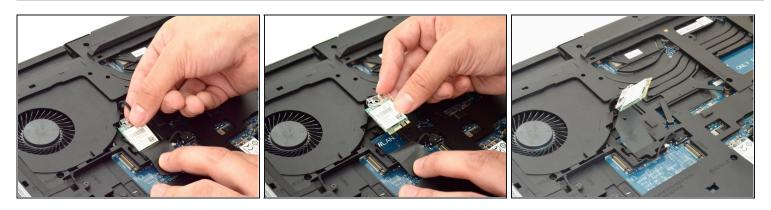
• Gently undo the clips attached to the wi-fi card.
