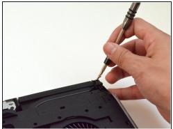
• Unscrew the **two M2x3 screws (1.9 mm)** at the top right and top left of the laptop that hold the tron lights in place.
