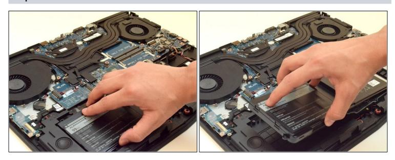
• Lift the battery up to remove it.
