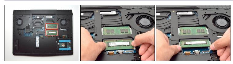
Move the metal sidings outward to release the RAM card.
