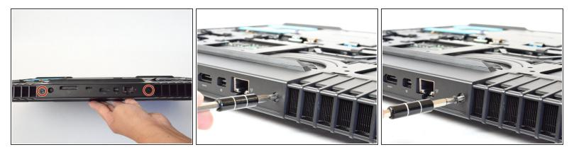
Remove the two M2.5x7 screws (2.44 mm) located on the rear panel using a PH1 screwdriver bit.
