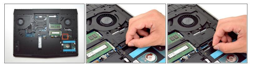
Disconnect the battery connector cable, located on the right side of the laptop, above the hard disk drive.
