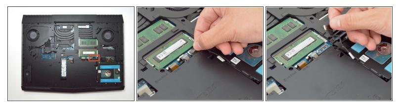
• **Gently** lift the HDD cable to disconnect it from the laptop.
