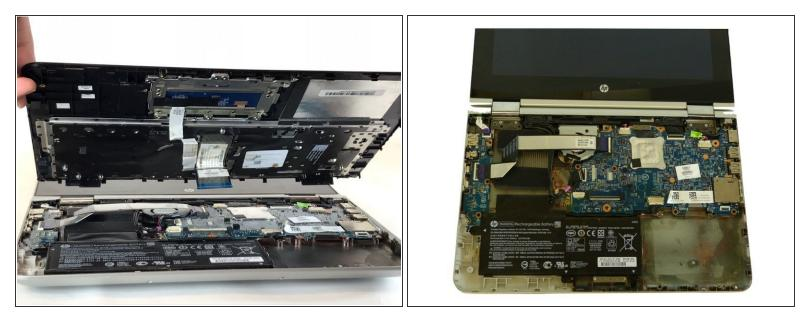
After the ribbon cables are disconnected, gently lift up the keyboard to disconnect it from the base of the laptop.
