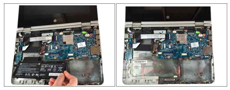
• Holding the lower right corner, gently lift up the battery to disconnect it from the motherboard.
