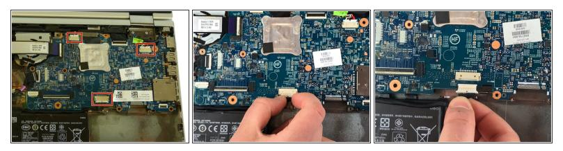
• Disconnect the 3 bundle cable connectors by gently gripping the cable wires and pulling outwards.
