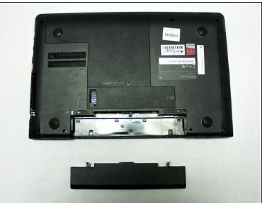
While holding the left and right lock switches in the unlock position, pull the battery away from the computer.
