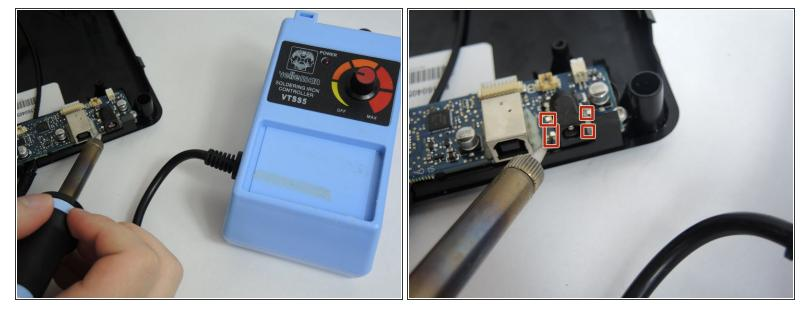
• To replace the power port, match the four contact points on the board to the new port and carefully solder the components together.
