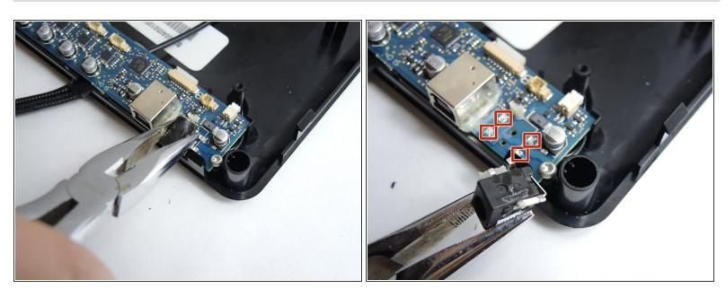
To remove the charging port grasp the port with a pair of pliers and use a soldering iron to desolder the joints at the red marks while carefully pulling away with the pliers.
