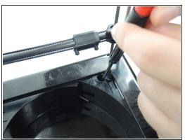
Remove the print bed cover and locate the four screws holding the print bed to the base of the unit.
