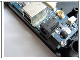
The ports are primarily soldered on to the board but are additionally secured using glue. Use the sharp metal spudger tool to gently pry apart the glue surrounding the ports.
