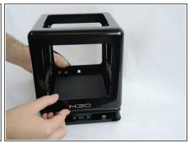
Place pressure on the central print bed and simultaneously pull up on the outer perimeter of the 3D printer. The cube shaped enclosure will lift up.
