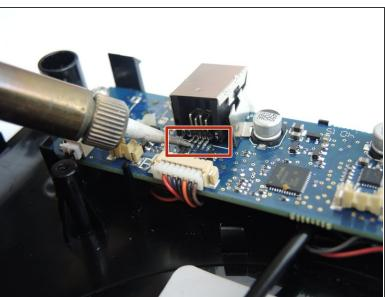
• To replace the USB data port, follow the same procedure as Step 5. The contact pins for the data port are on the back. The red marker indicates the four contact pins that must be matched up and carefully soldered on.
