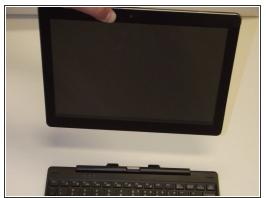
Remove the top section by pushing the middle button in the center of the base and lift on the screen.
