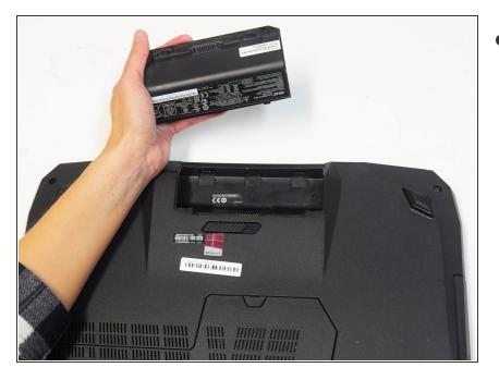
Remove the battery from its compartment.
