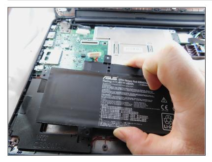
• Remove the battery from the bottom housing.
