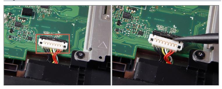
Disconnect the bundled cable connector that attaches the battery to the motherboard using the small plastic spudger.
