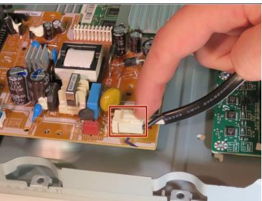
To remove the power cord, gently apply pressure to the tab located at the base of the cord and lift the cord with your fingers.
