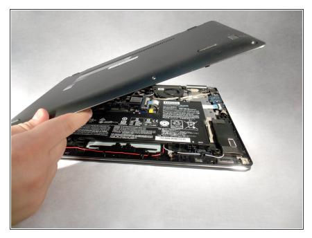
• Lift and remove the back cover.
