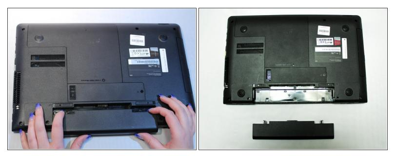
While holding the left and right lock switches in the unlock position, pull the battery away from the computer.
